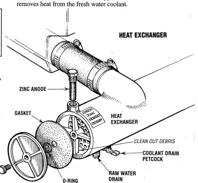
The heat exchanger is a copper cylinder which encloses a
