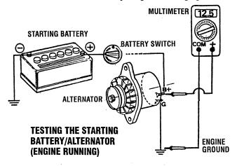
Start the engine again. Check the voltage between the alternator output and ground.
