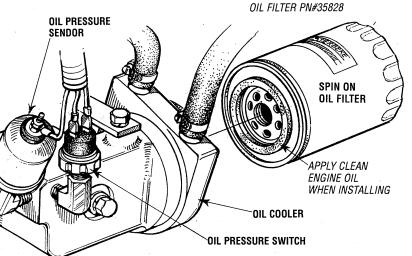
**NOTE:** Generic filters are not recommended, as the material standards or diameters of important items on generic parts might be entirely different from genuine parts. Immediately after an oil filter change and oil fill, run the engine to make sure the oil pressure is normal and that there are no oil leaks around the new oil filter.
