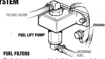
The fuel injection pump and the fuel injectors are precisely manufactured and they must receive clean diesel fuel, free from water and dirt. To ensure this flow of clean fuel, the fuel must pass through at least two fuel filters, a fuel filter/water separator and the engine's spin-on fuel filter. Visually inspect, clean, and change these filters according to the maintenance schedule in this manual.
