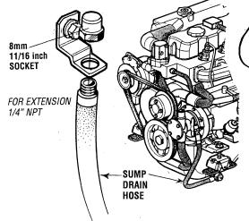
2. Replacing the Oil Filter. When removing the used oil filter, you may find it helpful and cleaner to punch a hole in the upper and lower portion of the old filter to drain the oil from it into a container before removing it. This helps to lessen spillage. A small automotive filter wrench should be helpful in removing the old oil filter.
