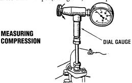
COMPRESSION PRESSURE STANDARD 427 psi at 200 rpm (30.0 kg/cm²)
