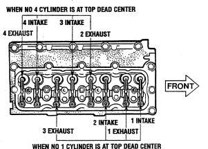
8. Adjust each valve's clearance by inserting a 0.012in (0.03mm) feeler gauge between the rocker arm and the valve stem. Make sure to adjust all valves when the engine is cold.
