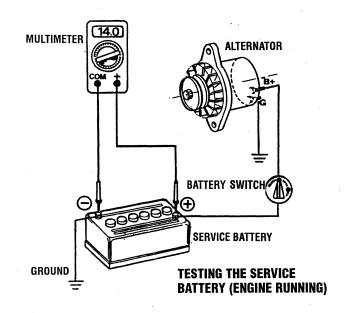
A CAUTION: To avoid damaging the alternator diodes, do not use a high voltage tester (i.e. a megger) when performing tests on the alternator charging circuit.
