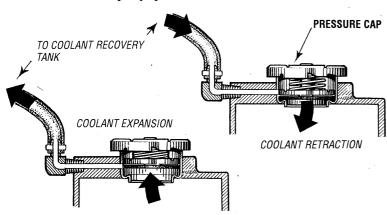
**NOTE:** Periodically check the condition of the manifold pressure cap. Ensure that the upper and lower rubber seals are in good condition and check that the vacuum valve opens and closes tightly. Carry a spare cap.
