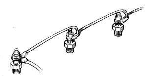
Re-install the plugs in the engine and test them again. The plugs should get very hot (at the terminal end) within 20 to 25 seconds. If the plugs don't heat up quickly, check for a short circuit. When reinstalling the glow plugs, use anti-seize compound on the threads.
