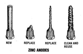
**NOTE:** Electrolysis action is the result of each particular installation and vessel location; not that of the engine.
