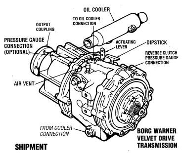
For safety reasons, the transmission is *not* filled with transmission fluid during shipment and the selector lever is temporarily attached to the actuating shaft.
