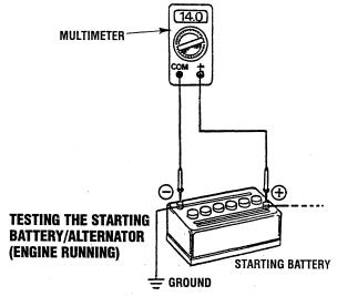
3. Turn off the engine. Inspect all wiring and connections. Ensure that the battery terminals and the engine ground connections are tight and clean.
